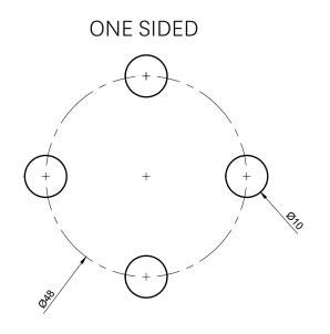
If handle is mounted on only one side, drill four 10mm holes.
