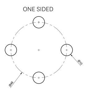
If handle is mounted on only one side, drill four 10mm holes.
