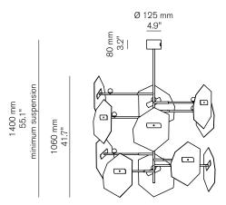
Brass. Diffuser Brass or Fibreglass
